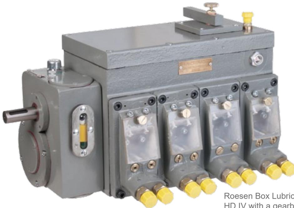
Roesen Box Lubricator system HD IV with a gearbox in pressure-tight version
